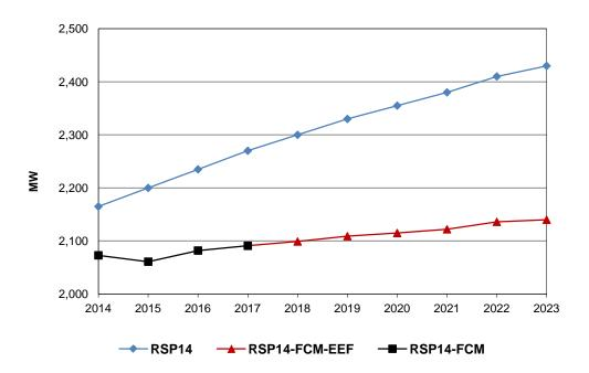
Figure 5-13: Summer peak demand forecast (90/10) for Rhode Island (diamond), load forecast minus FCM #8 results through 2017 (square), and load forecast minus FCM results and minus the energy-efficiency forecast (triangle) for 2018 to 2023 (MW).
