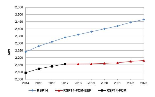
Figure 5-9: Summer peak demand forecast (90/10) for Maine (diamond), load forecast minus FCM #8 results through 2017 (square), and load forecast minus FCM results and minus the energy-efficiency forecast (triangle) for 2018 to 2023 (MW).
