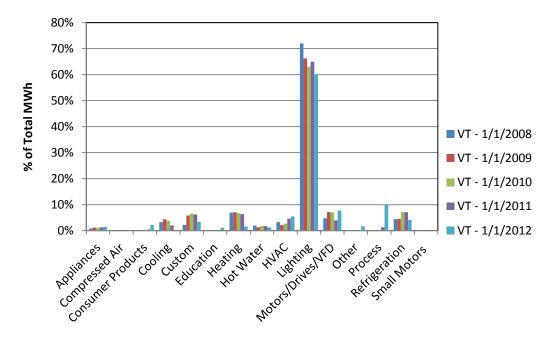
Figure 7-11: Percentage contributions to energy savings (MWh) in Vermont by various measures, 2008 to 2012.
