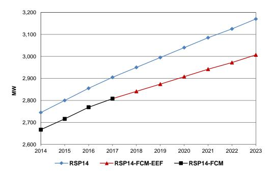
Figure 5-11: Summer peak demand forecast (90/10) for New Hampshire (diamond), load forecast minus FCM #8 results through 2017 (square), and load forecast minus FCM results and minus the energy-efficiency forecast (triangle) for 2018 to 2023 (MW).
