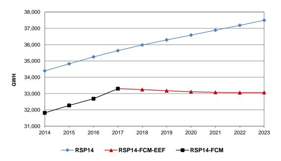
Figure 5-4: Net energy-use load forecast for Connecticut (diamond), net energy-use load forecast minus FCM #8 results through 2017 (square), and load forecast minus FCM results and minus the energy-efficiency forecast (triangle) for 2018 to 2023 (GWh).
