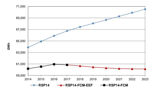
Figure 5-6: Net energy-use load forecast for Massachusetts (diamond), net energy-use load forecast minus FCM #8 results through 2017 (square), and load forecast minus FCM results and minus the energy-efficiency forecast (triangle) for 2018 to 2023 (GWh).
