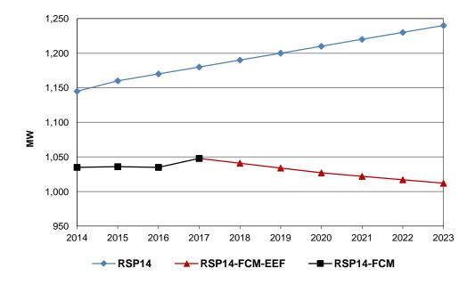
Figure 5-15: Summer peak demand forecast (90/10) for Vermont (diamond), load forecast minus FCM #8 results through 2017 (square), and load forecast minus FCM results and minus the energy-efficiency forecast (triangle) for 2018 to 2023 (MW).
