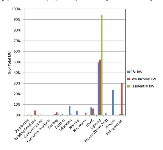
Figure 7-3: Percentage of demand (KW) in New England, by type of energy-efficiency measure and sector, total for 2009 to 2011.
