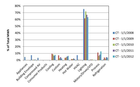
Figure 7-5: Percentage contributions to energy savings (MWh) in Connecticut by various measures, 2008 to 2012.
