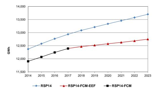
Figure 5-10: Net energy-use load forecast for New Hampshire (diamond), net energy-use load forecast minus FCM #8 results through 2017 (square), and load forecast minus FCM results and minus the energy-efficiency forecast (triangle) for 2018 to 2023 (GWh).
