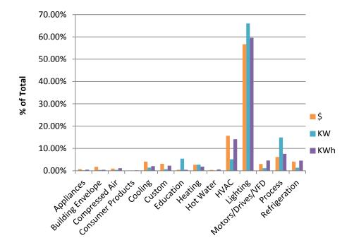
Figure 7-1: Percentage of costs (\$), demand (kW), and energy use (KWh), for each type of energy-efficiency measure used by programs in the New England states, total for 2009 to 2012.
