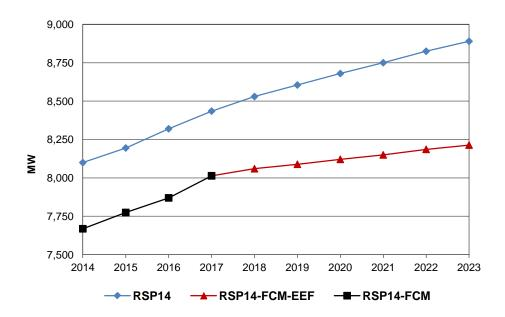
Figure 5-5: Summer peak demand forecast (90/10) for Connecticut (diamond), load forecast minus FCM #8 results through 2017 (square), and load forecast minus FCM results and minus the energy-efficiency forecast (triangle) for 2018 to 2023 (MW).
