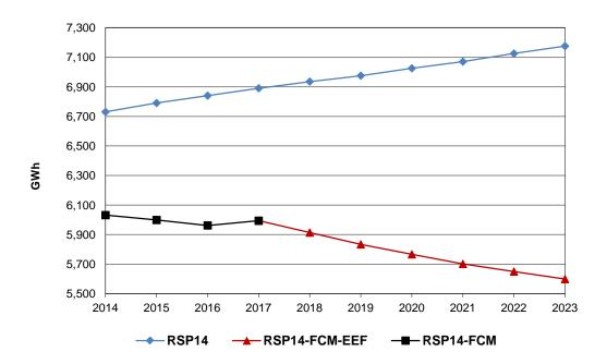
Figure 5-14: Net energy-use load forecast for Vermont (diamond), net energy-use load forecast minus FCM #8 results through 2017 (square), and load forecast minus FCM results and minus the energy-efficiency forecast (triangle) for 2018 to 2023 (GWh).
