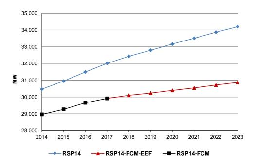
Figure 5-2: Summer peak demand forecast (90/10) (diamond), load forecast minus FCM #8 results through 2017 (square), and load forecast minus FCM results and minus the energy-efficiency forecast (triangle) for 2018 to 2023 (MW).
