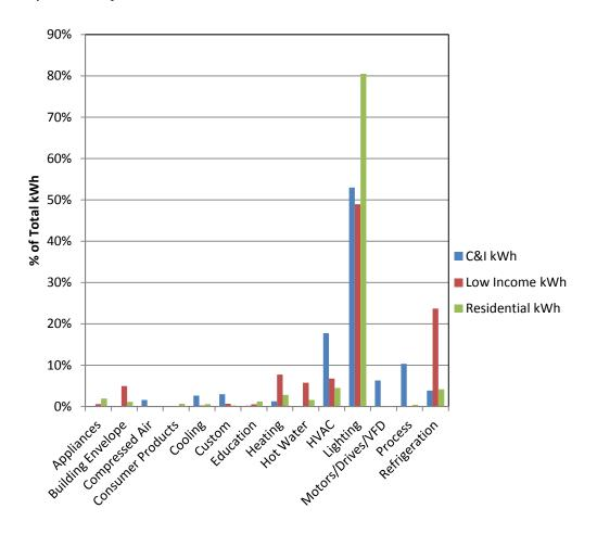
Figure 7-2: Percentage of energy use (kWh) in New England, by type of energy-efficiency measure and sector, total for 2009 to 2011.
