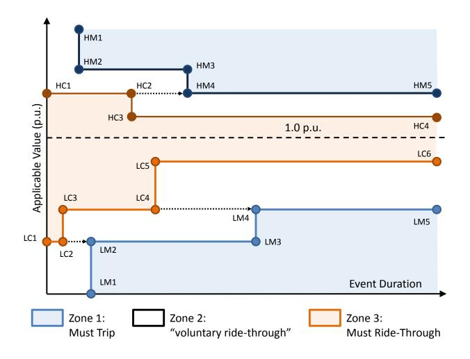
Voltage Ride-through – ISO recommendation is to establish a minimum time for inverter-based generation to stay connected after IEEE 1547 is revised – until then use 1547a
