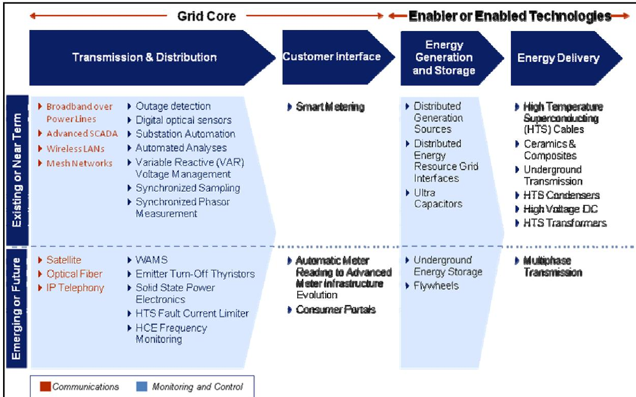
**Figure 4: Existing and emerging Smart Grid communications and monitoring and control technologies in the electricity supply chain.**
