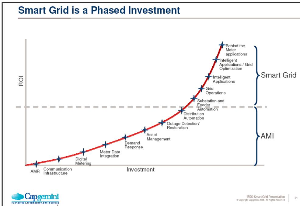
**Figure 6: The phased return on investments from advanced metering infrastructure to Smart Grid.**
