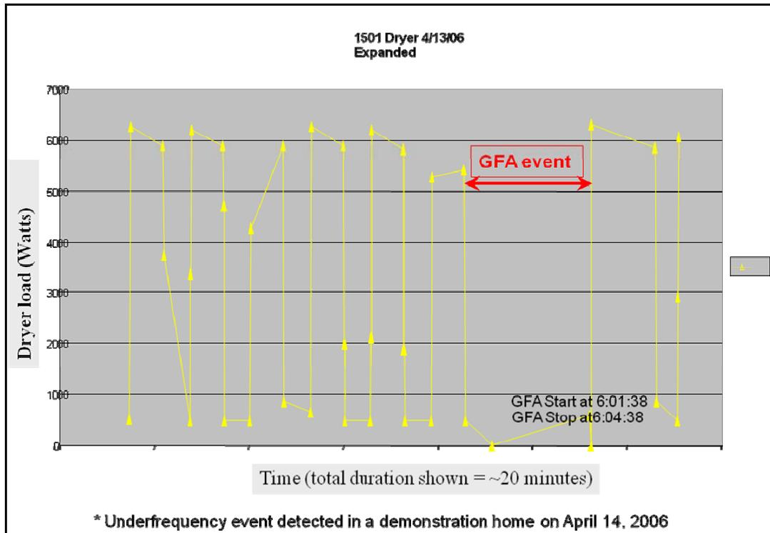
**Figure 8: GFA voltage-frequency event.**
