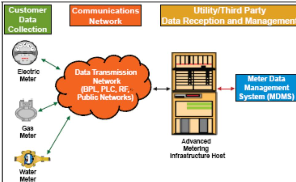
**Figure 5: Building blocks for advanced metering interfaces.**
