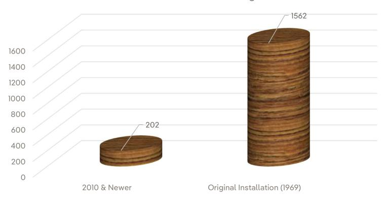
This figure illustrates that regular structure maintenance/replacements started in 2010. The majority of poles date back to the original installation in 1969 (approximately 54 years of age).
