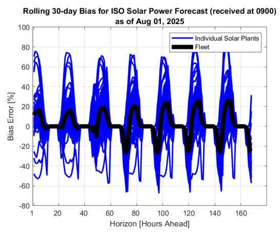
Ideally, MAE and Bias would be both equal to zero. Positive bias means less solar power was actually available compared to forecast. Negative bias means more solar power was actually available compared to forecast.
