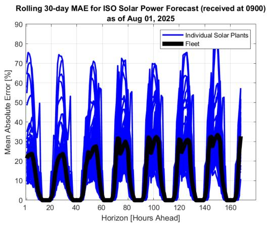
Ideally, MAE and Bias would be both equal to zero. As is typical, MAE generally increases with the forecast horizon. MAE and Bias for the fleet of solar power resources are less due to offsetting errors.
