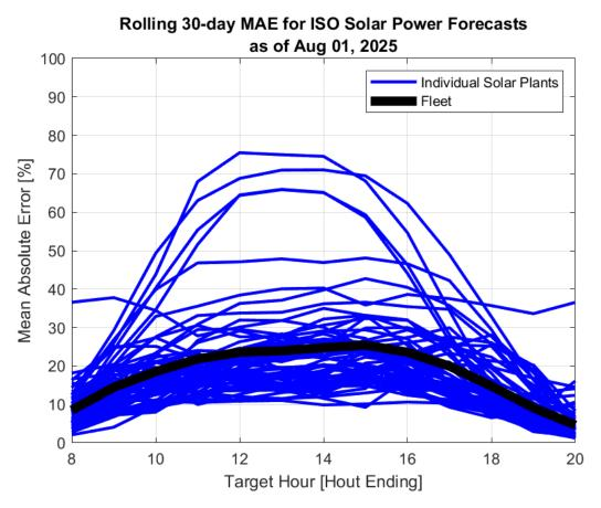
Ideally, MAE and Bias would be both equal to zero. Typically, MAE increases with the forecast horizon. As shown, MAE also generally increases with expected power output. MAE and Bias for the fleet of solar power resources are less due to offsetting errors.
