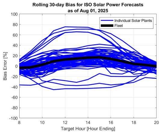
Ideally, MAE and Bias would be both equal to zero. Positive bias means less solar power was actually available compared to forecast. Negative bias means more solar power was actually available compared to forecast.
