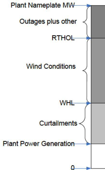
Curtailed operation means that the plant is being actively controlled (whether manually or automatically) to reduce output to below the maximum amount of power that could be produced by the available equipment given the current weather conditions. Curtailment specifically excludes the effects of physical conditions such as wind speed and/or icing conditions.
