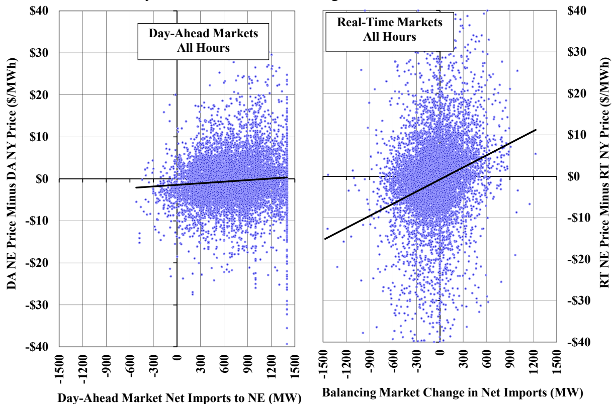
Figure 10: Efficiency of Scheduling in the Day-Ahead and Real-Time Primary Interface Between New England and New York, 2016
