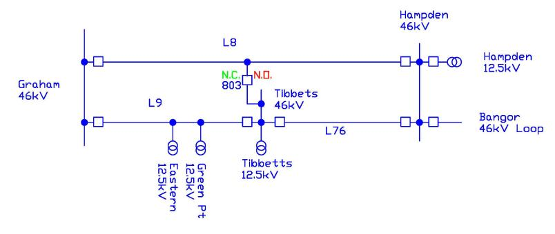
Update protection on Line 8 and add communications to allow the circuit to operate as three terminal, with Bkr 803 closed.
