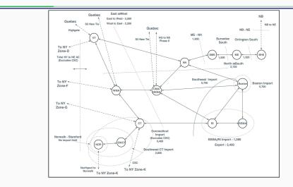
The zonal network model consists of 13 RSP zones with 21 interfaces and tie-lines.
