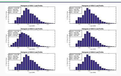
2030 Scenario load distributions exhibit the same statistical characteristics except Scenario 3 due to the addition of energy efficiency and electric vehicles.
