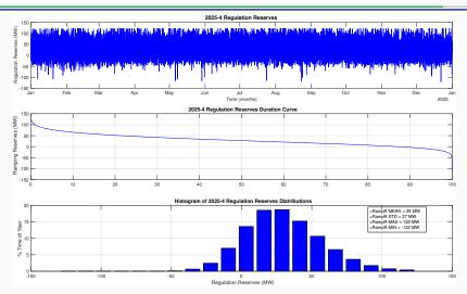
Scenario 2025-4 shows a balanced usage of regulation. Saturation does not appear to occur in any of three figures.
