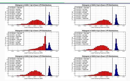
Scenario 2025-3 shows a shortage of downward load following reserves reflecting constrained downward dispatch.
