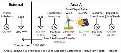
600 MW + (1440 MW + 520 MW) - 500 MW + 10 MW = 990 MW + 1080 MW 2070 MW = 2070 MW
