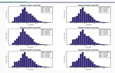
2025 Scenario load distributions exhibit the same statistical characteristics except Scenario 3 due to the addition of energy efficiency and electric vehicle charging loads.
