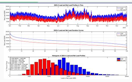
Variable resources create lower net load curve. Dispatchable resources must meet new variability, min load, & retain peak load capability.
