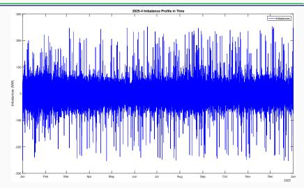
Imbalances are well-controlled to zero mean and moderate variability on the order of 75MW for the overwhelming majority of the year.
