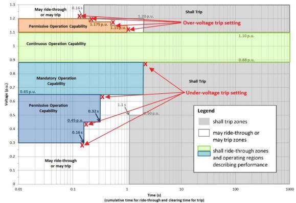
Voltage trip settings and voltage ride-through settings used for 2018 DERs align with IEEE Std 1547-2018 and ISO Source Requirement Document
