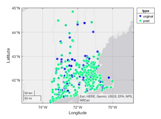
Green dots: DER tripped in this simulation Blue dots: DER tripped in the original minimum load case (on slide 13), but not in this simulation
