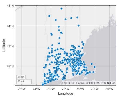
Each blue dot represents a substation where DER solar generation was tripped. DER in the New York system was not explicitly modeled.
