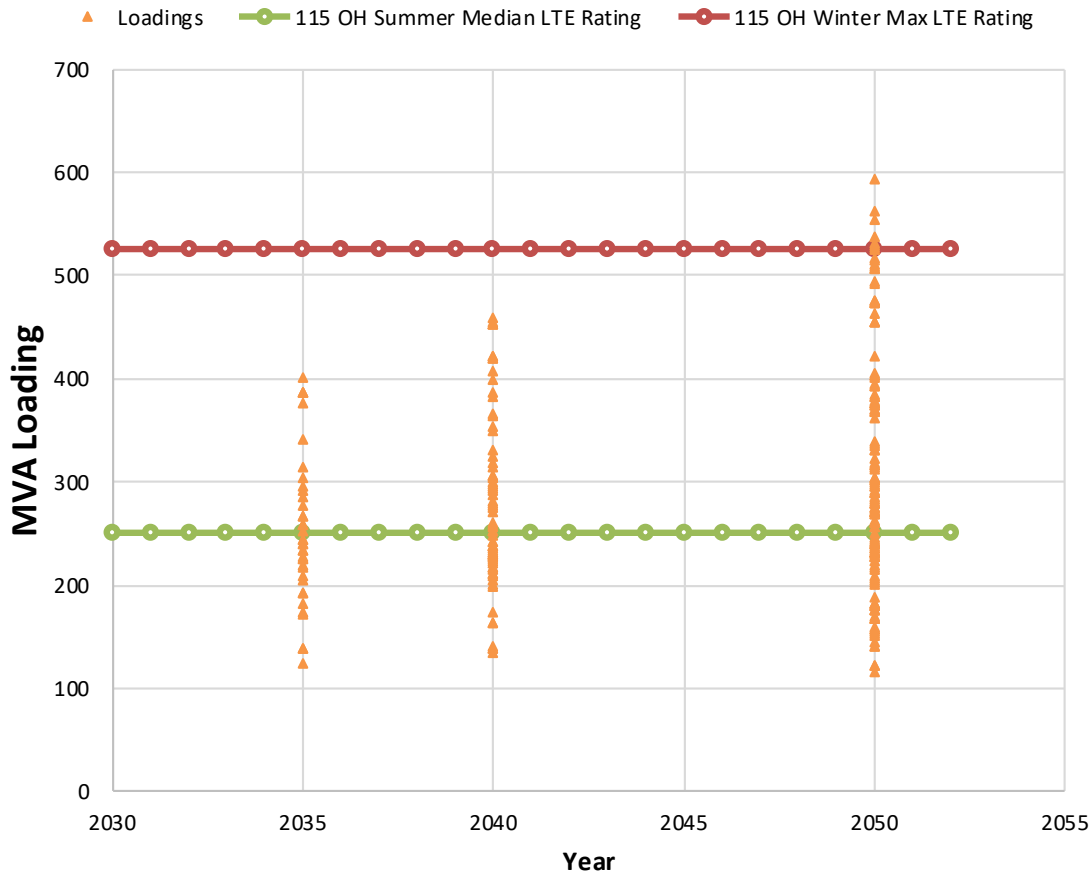
115 kV Overhead Maximum MVA Flows Summer
