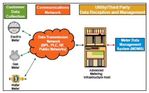
Figure 5: Building blocks for advanced metering interfaces. Source: FERC, 2007 (FERC-1)
