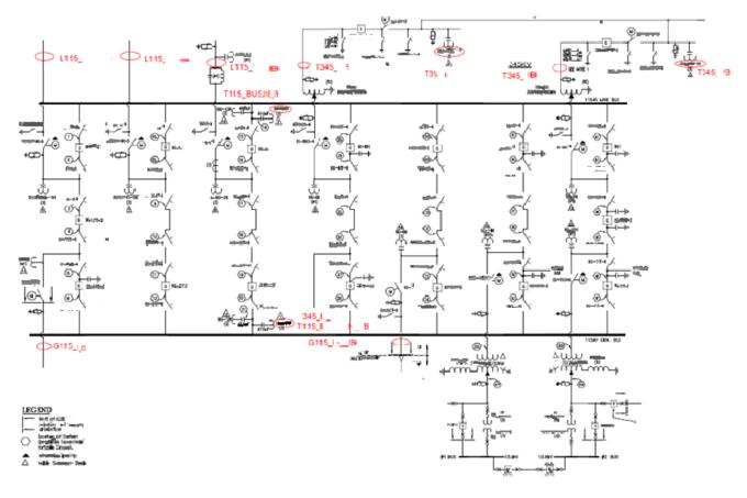
Figure 1 – Sample One-Line Drawing with PMU Inputs (intentionally blurred nomenclature for public release)
