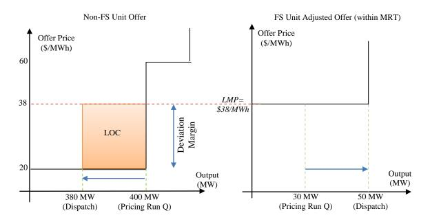
Figure 1- Calculation of the lost opportunity cost (LOC) in Example 1, for the non-fast start unit during the first 30 minutes of the fast-start unit's operation
