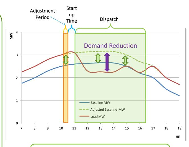
Note that at the 30 minute point in this example (10:59), the load = the adjusted baseline, so based on this dispatch, this asset was not capable of providing 30 minute reserves.
